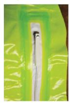
If the zipper is **black with plastic teeth**, use Molykote<sup>™</sup> 33 Light lubricant. If the zipper is **white with bright metal teeth** apply paraffin wax lightly on the teeth of the closure while open. After lubricant is applied, close and open the zipper several times to ensure smooth function and to remove excess lubricant.
