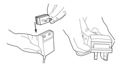
Connect the batteries to the chargers, as shown below, and with chargers plugged into a 120V electrical outlets. Charge batteries.
