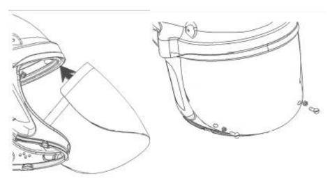
Ensure both securing screws and nuts are fitted.
