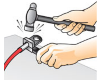
*Swedge-on process The swedge-on tool provides an easy and convenient way to install BLUESHIELD™ cable lugs and cable splicers to welding cable. Insert bare cable strands into the lug barrel and impact with the swedge tool as shown in the illustration.
