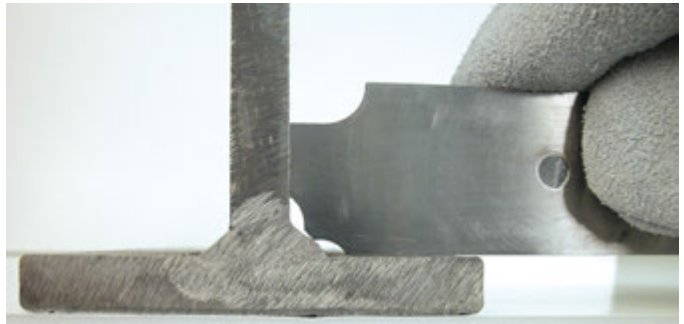
2. CHECKING FILLET WELD THROAT SIZE
