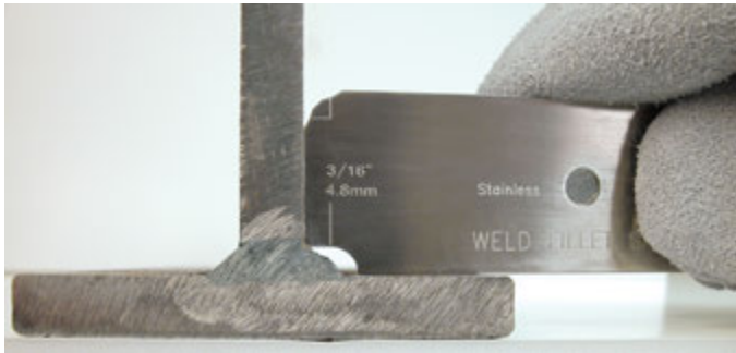
1. CHECKING FILLET LEG SIZE
