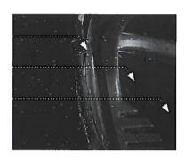
Hydrophobic Action Water droplets form and are repelled to the sides of the lens.
