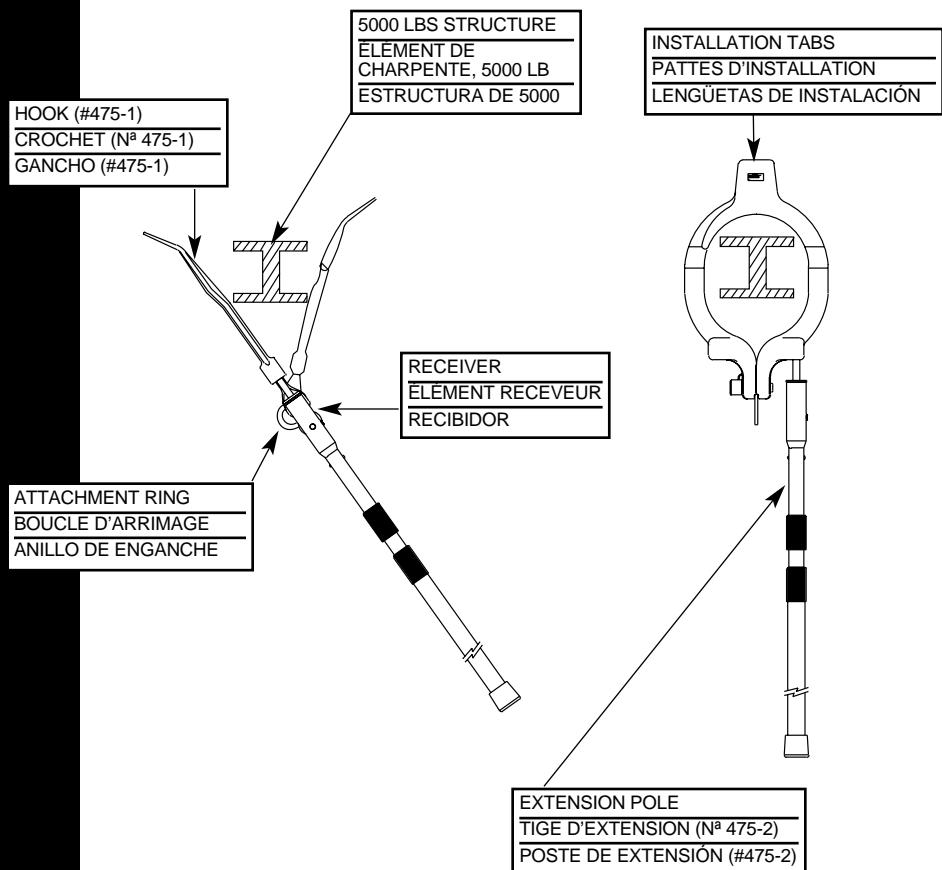
4. Install the hook by pushing it over the anchorage and rotating it 90 degrees. Both halves of the hook must come together for proper attachment to the anchorage. Examples of such anchorages may be small beams, angle or other structures that the device will accommodate and maintain a 5,000 lbs. tensile strength.
